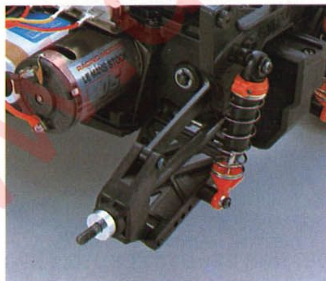
REAR SUSPENSION (SAME DESIGN). RELIABLE FRICTION SHOCK. ADJUSTABLE SHOCK MOUNTS.
